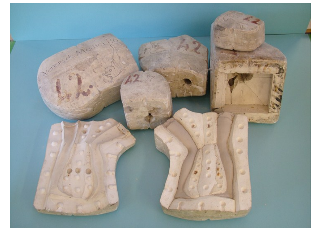
Example of a group of piece-moulds for porcelain reproduction of “Venus de’ Medici” statue.
